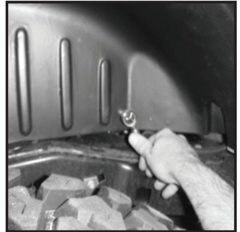
5. Secure the axle vent hose with the Wheel Liner mounting hardware on the rear passenger side. There is a hole in the plastic clip attached to the hose for making the attachment. The hose should be secured to the rear most mounting hole in the Wheel Liner just above the frame rail.
